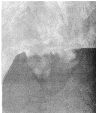
Figure 4.26 TEM image (enlarged): Poly-Si has entered through damaged gate oxide film.
